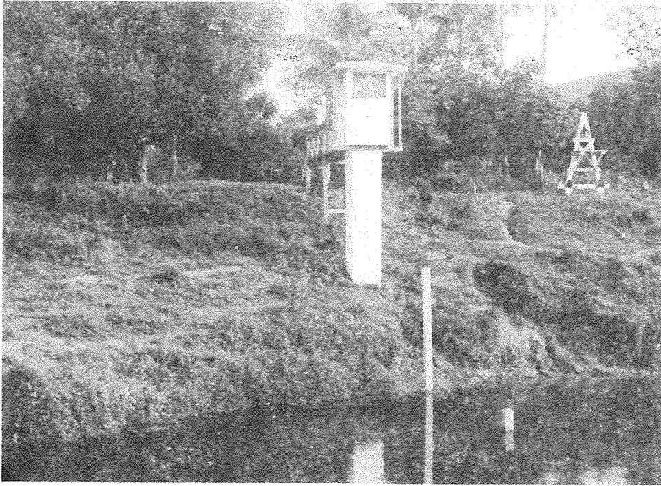
Figure 3. Recording Gaging Station of Lam Takhong at Ban Khlong Phai (M. 38C) Nakhon Ratchasima.
